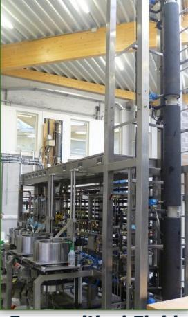
Supercritical Fluid Extractors SFE-CO<sub>2</sub>
